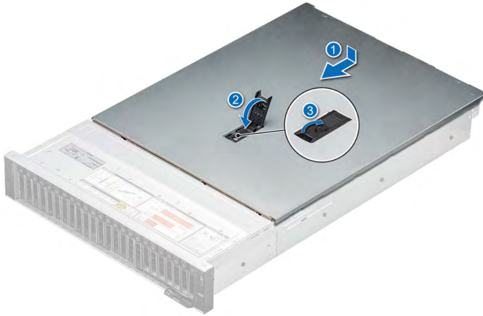
Figure 58. Installing the system cover
