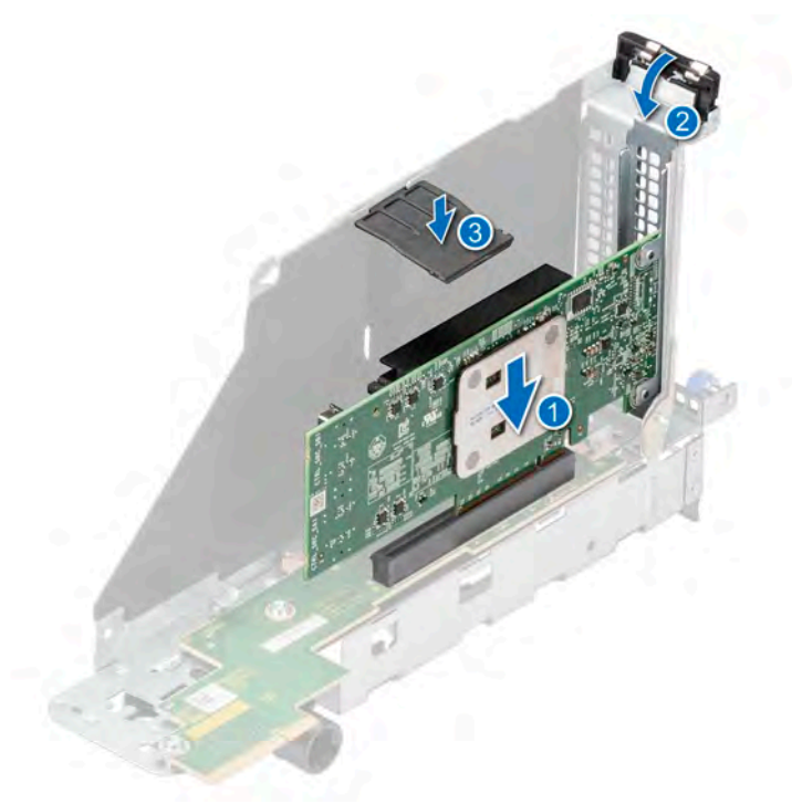
Figure 102. Installing the APERC module
