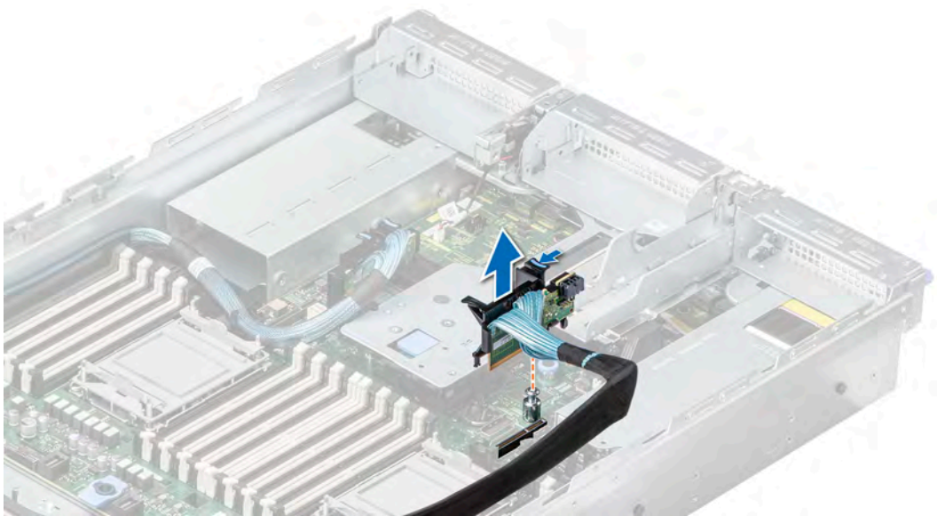
Figure 167. Removing the R1 paddle card
