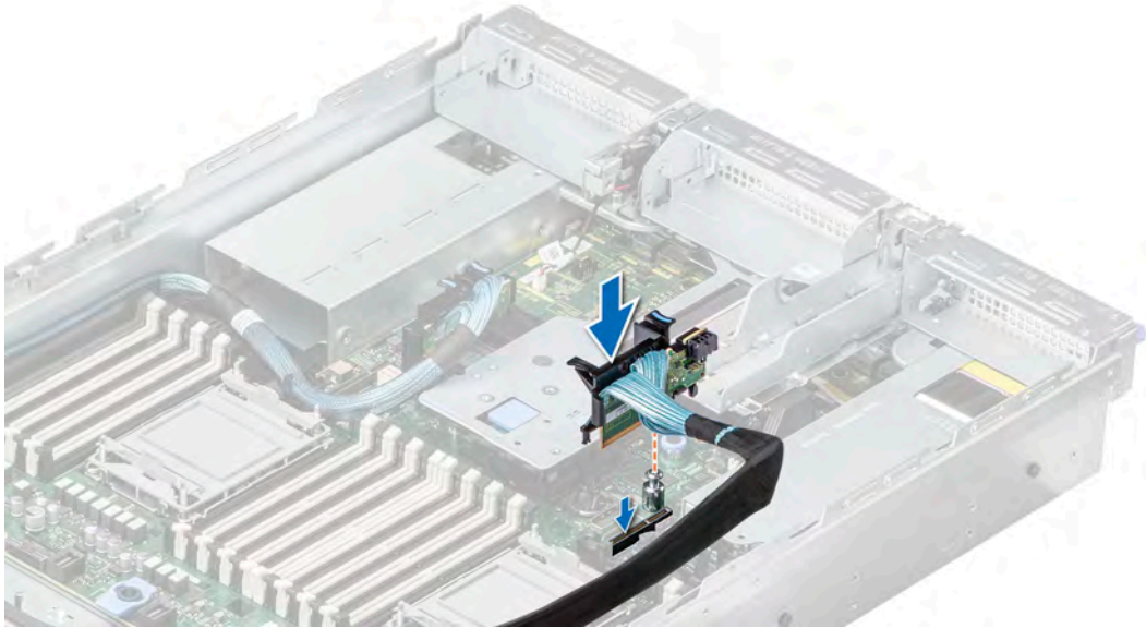
Figure 169. Installing the R1 paddle card
