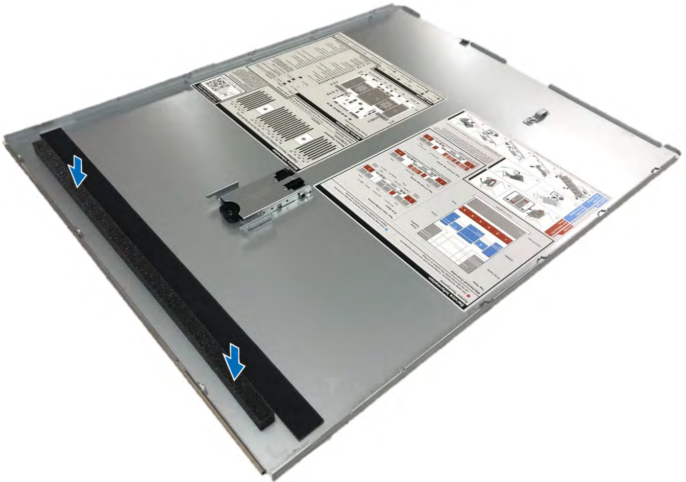
Figure 224. Installing Mylar foam on the system cover
