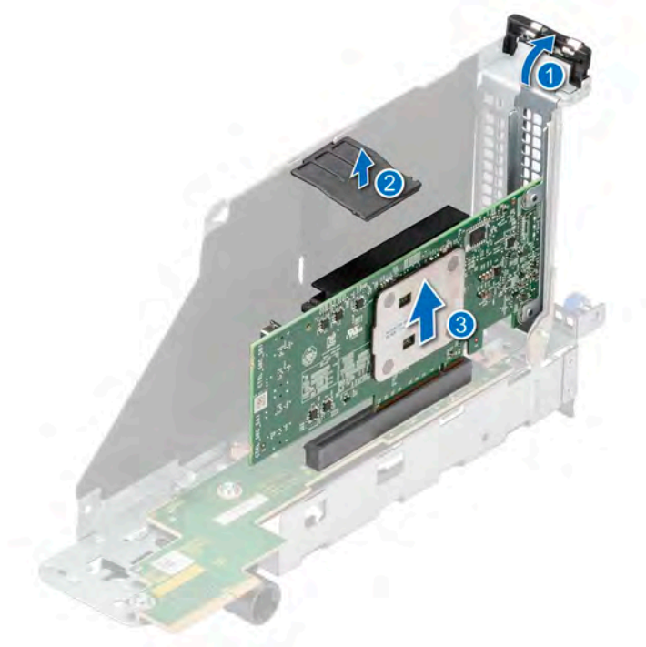
Figure 99. Removing the APERC module
