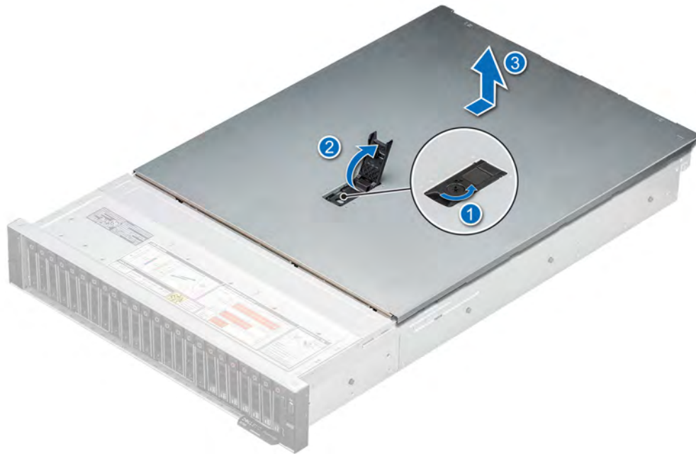
Figure 57. Removing the system cover
