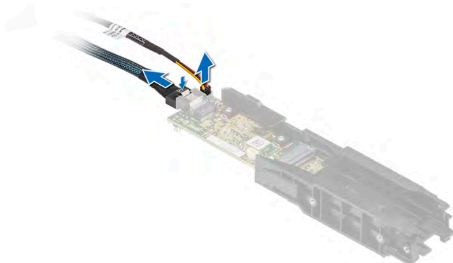
Figure 190. Removing the BOSS S2 power and signal cable from the BOSS S2 module
