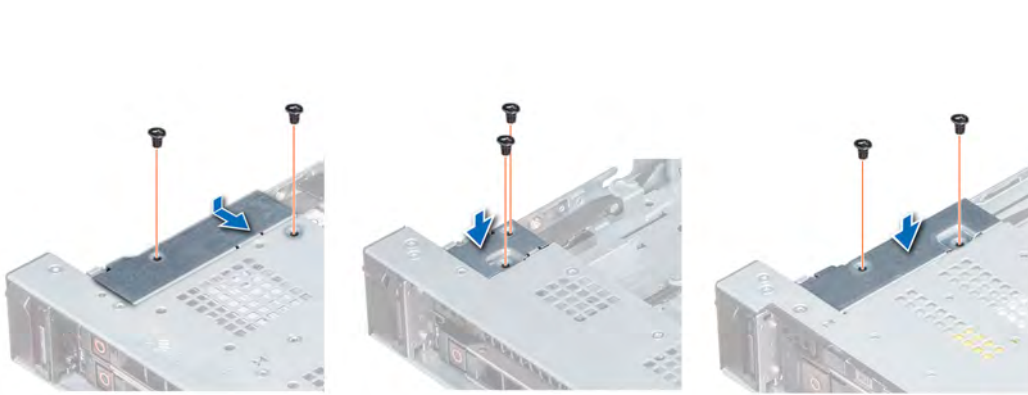
Figure 115. Installing the cable cover
