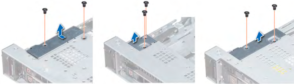
Figure 112. Removing the cable cover
