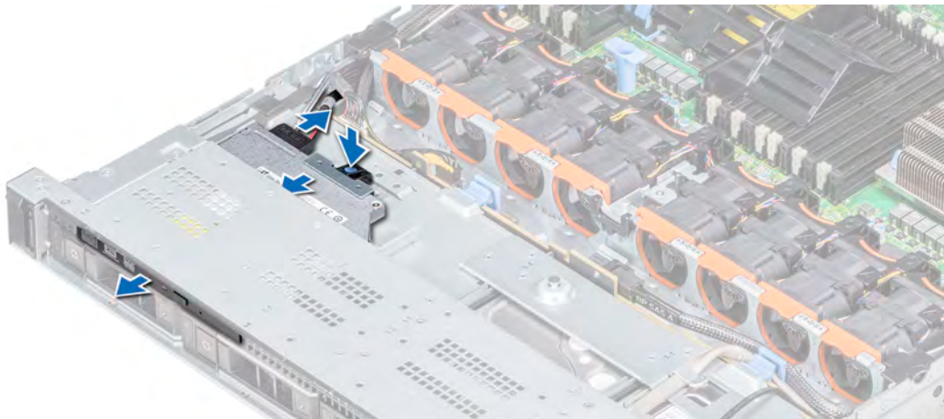
Figure 103. Removing optical drive
