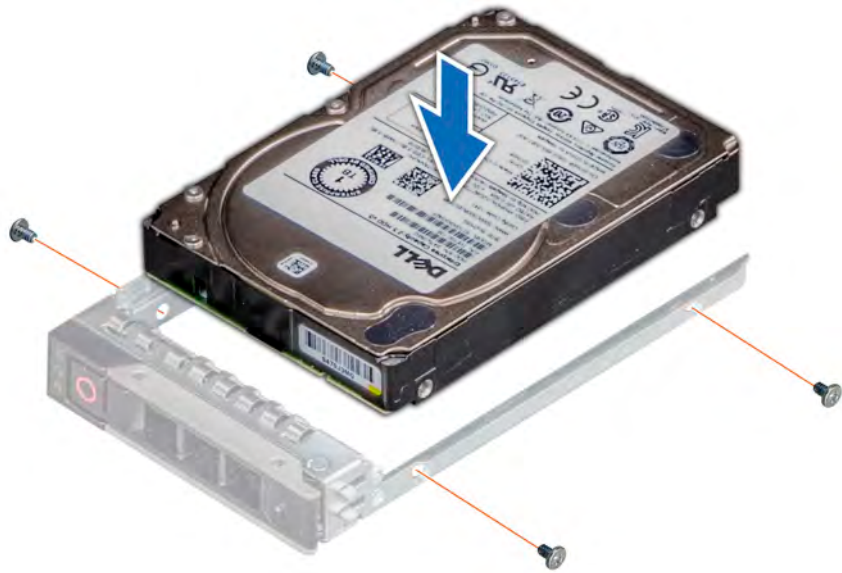
Figure 78. Installing a drive into the drive carrier
