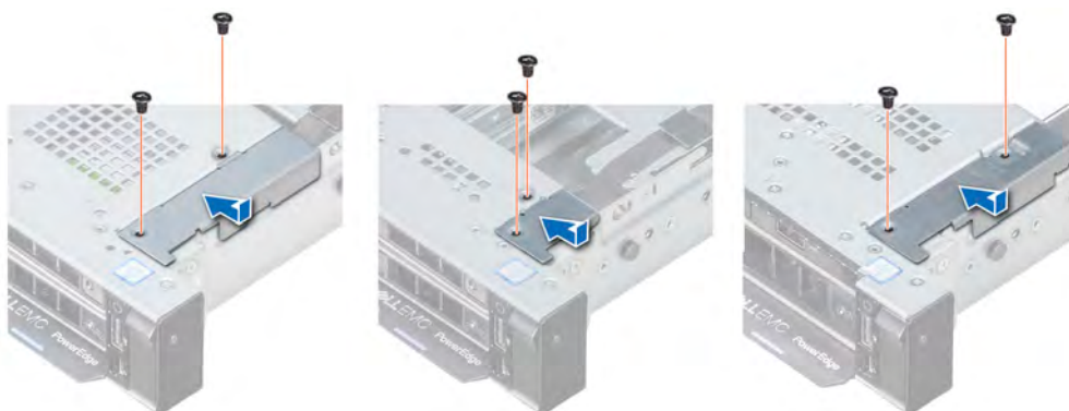
Figure 119. Installing the cable cover
