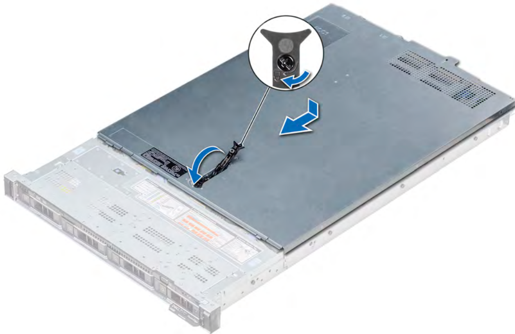
Figure 23. Installing the system cover
