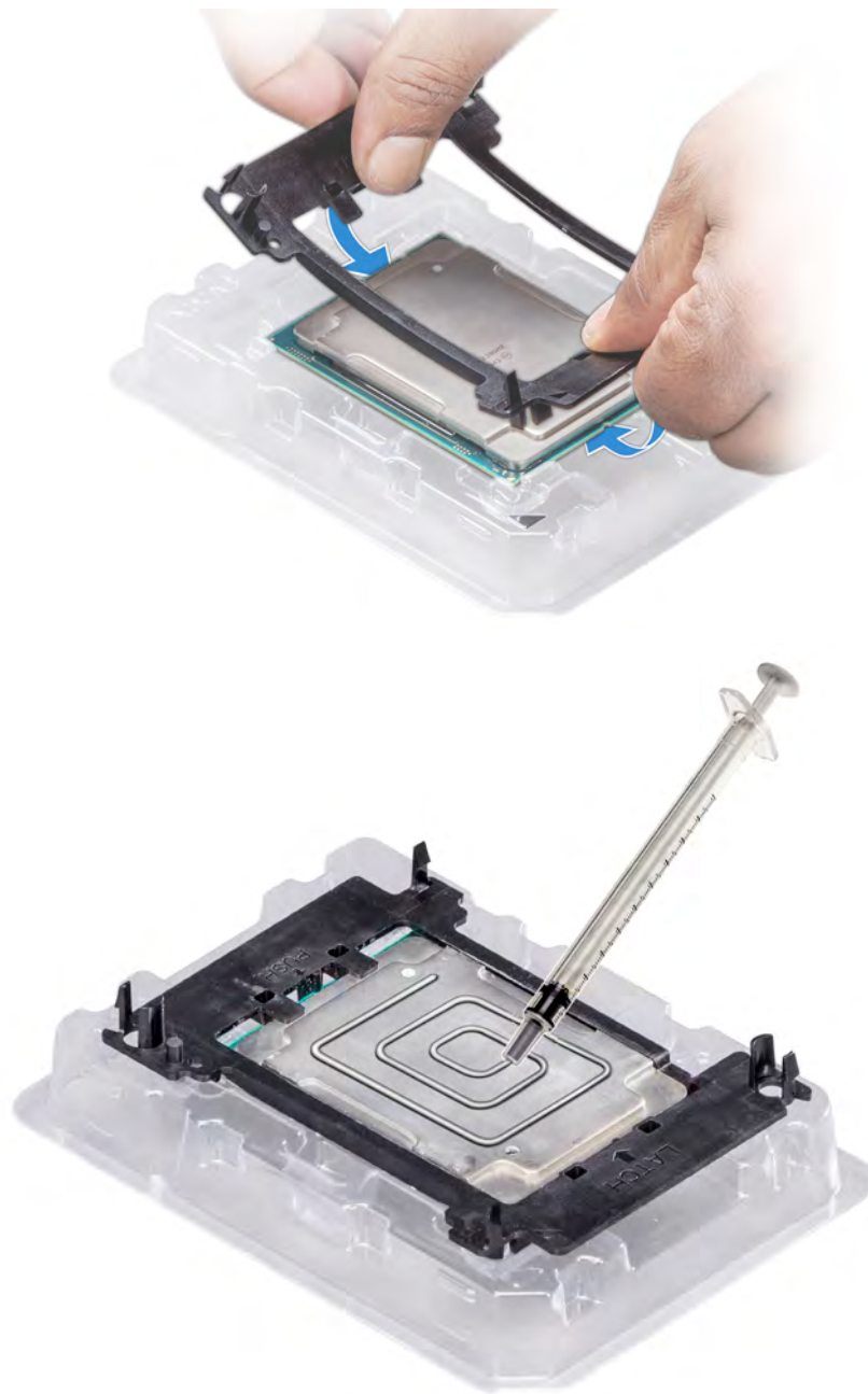
Figure 43. Applying thermal grease on top of the processor
