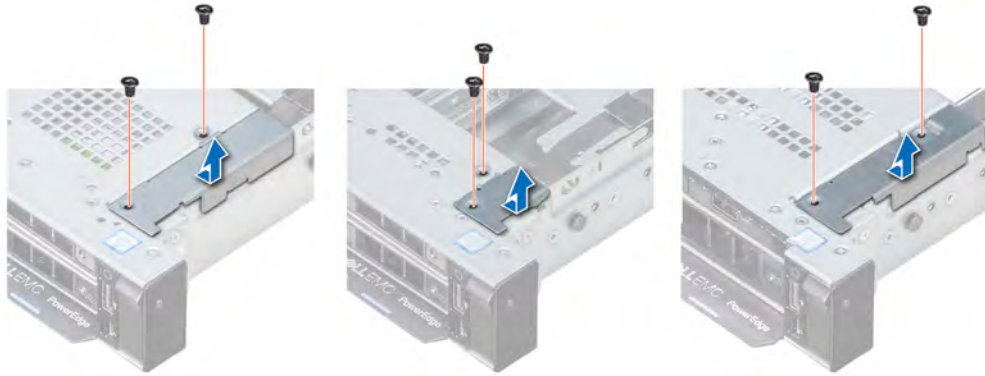
Figure 116. Removing the cable cover
