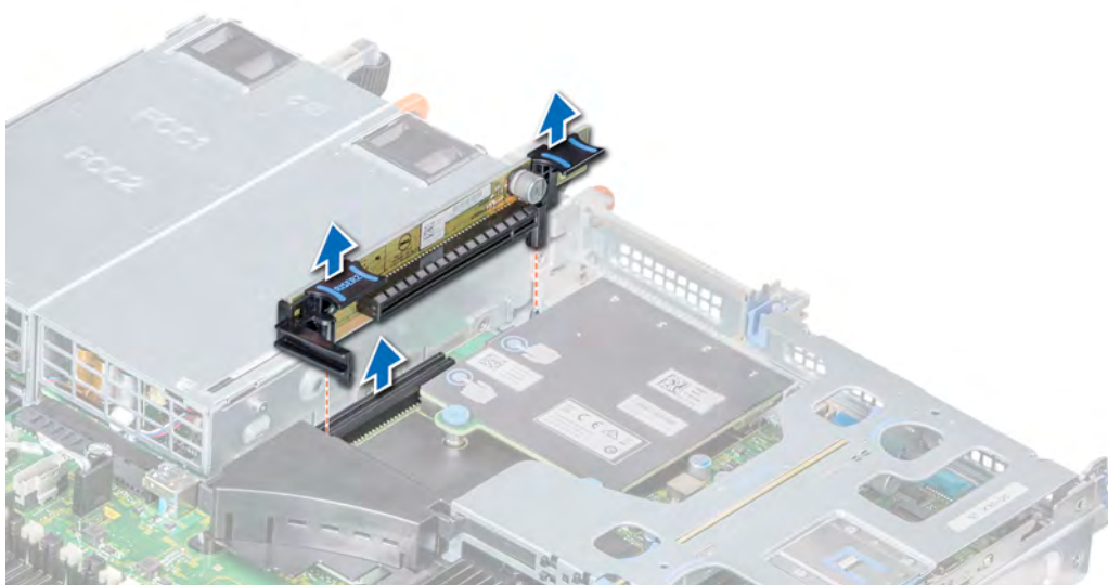
Figure 48. Removing the expansion riser 2A
