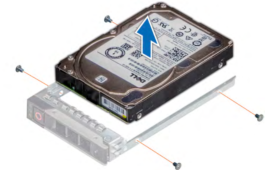
Figure 77. Removing the drive from the drive carrier
