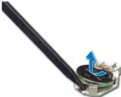
Figure 97. Removing the system battery
