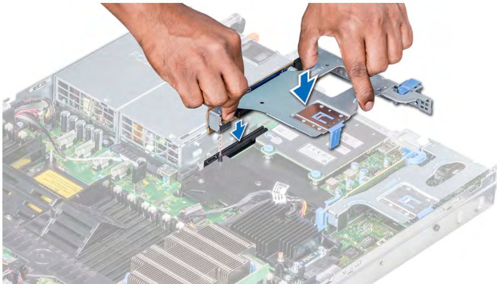
Figure 53. Installing the expansion riser 2B
