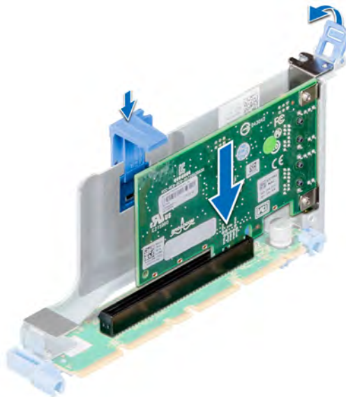
Figure 60. Installing an expansion card into the expansion riser 1B
