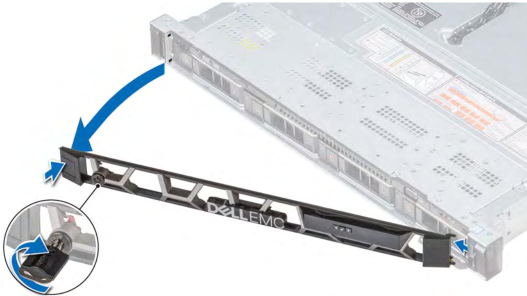
Figure 20. Removing the optional front bezel with the LCD panel
