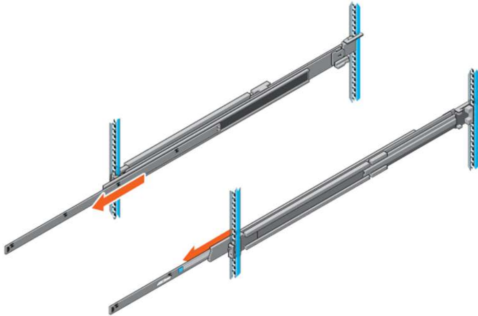
Figure 18. Pull out inner rail
