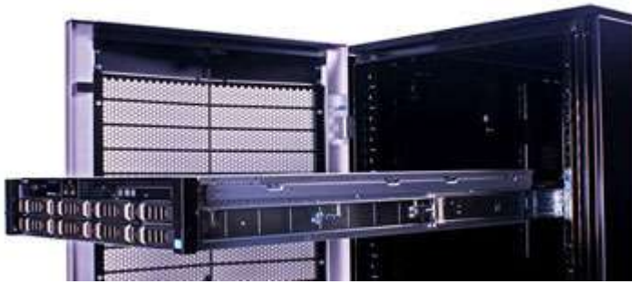
Figure 17. Sliding rails with CMA
