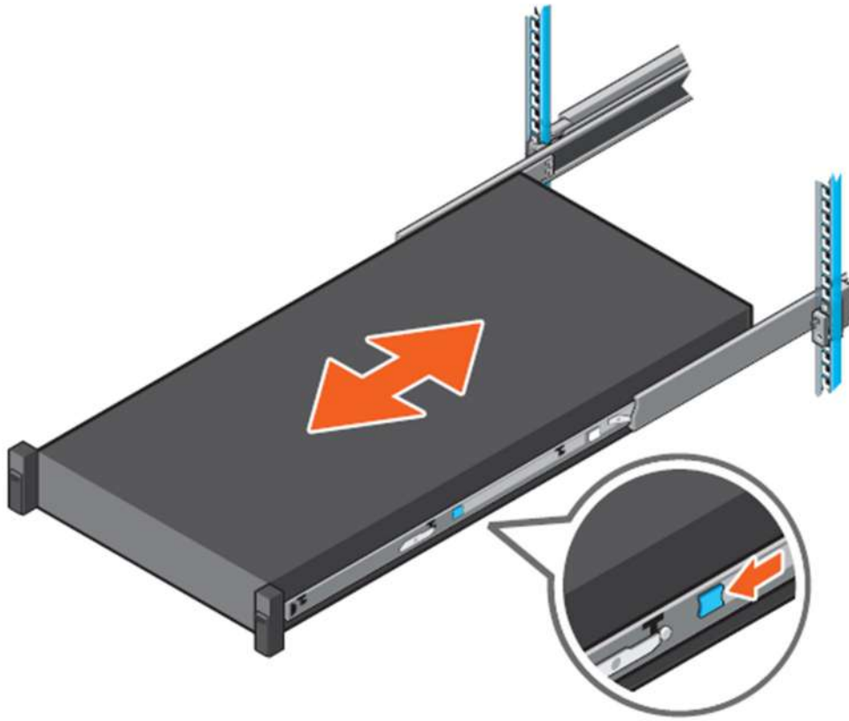
Figure 20. Slide system into the rack
